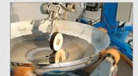
Polishing of a stainless steel head
