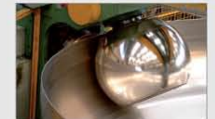
Flanging process of a stainless steel head
